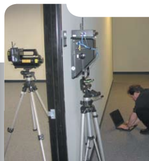
RTR-4 can be used for wall inspections.
