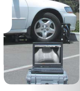
RTR-4 set up for inspection of car tire.
