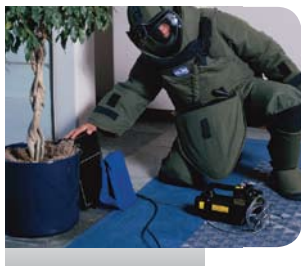
Bomb squad technician sets up RTR-4 to acquire image of suspicious object in a typical office lobby.
