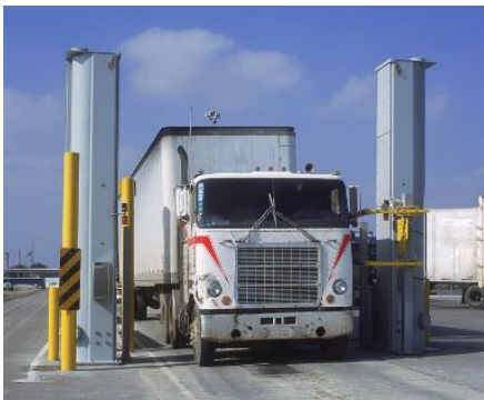
The Portal VACIS system scans containers with minimal impact on the flow of traffic.
