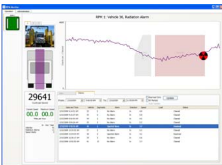
The SRM-910 RPM graphically displays the location of radioactive sources in scanned vehicles.
