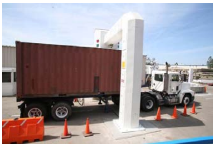
The VACIS IP6500 system performs x-ray imaging and spectroscopic radiation detection in the typical flow of checkpoint traffic.
